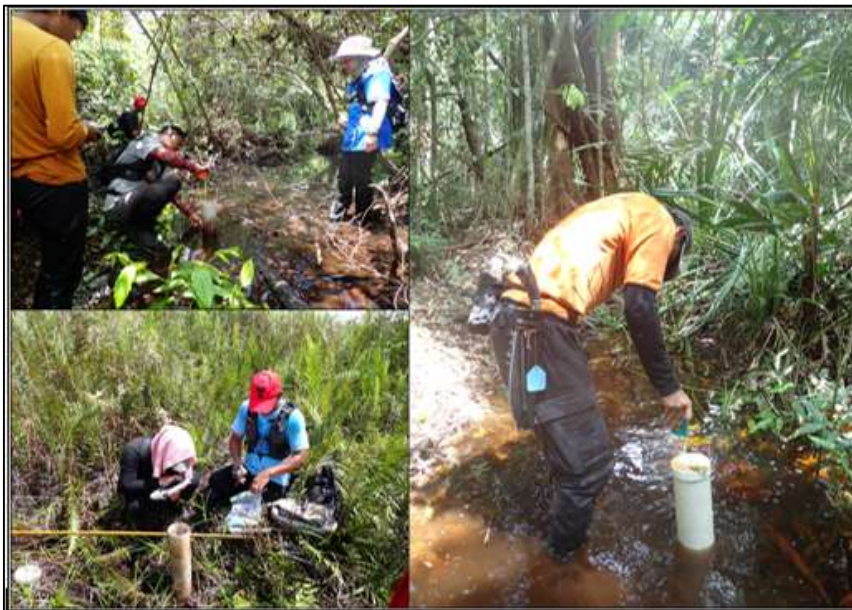
Figure 9: Joint piezometer data collection by FERT and Forest Protection teams at Pekan West FR using manual readings and HOBO logger data extraction
