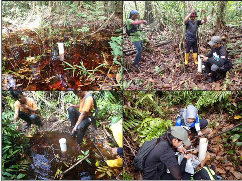
Figure 8: Piezometer data collection at Pekan East FR with manual measurement and HOBO automatic data logger
