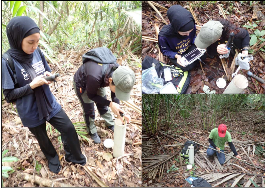
Figure 10: Forest Protection team marking coordinates (integrated with SMART Patrolling), preparing ROG for HOBOL logger data extraction, and manually measuring water table level as reference at Nenasi FR
