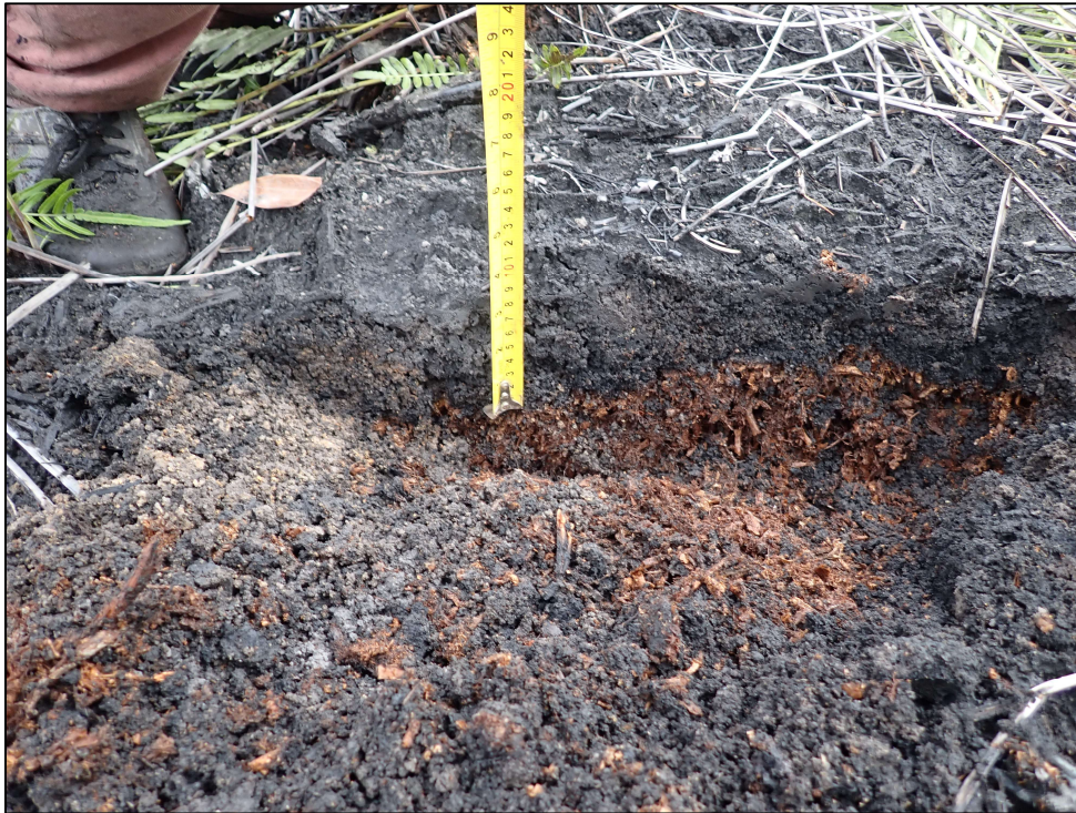
Figure 6: Measurement of peat burnt scar depth using a measuring tape, based on visual identification of the boundary between burned and unburned peat layers
